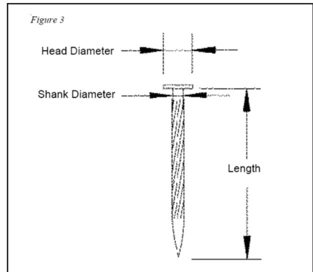
Pneumatically driven pins are proprietary products that have unique characteristics and performance capabilities that vary by manufacturer. Pin manufacturers publish design values for their own products, typically in a format similar to nailing schedules. Consult individual pin manufacturers for design values for their specific products.
