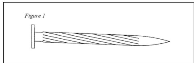
friction. An increase in stud thickness or tensile strength will increase the pin's pullout resistance.
